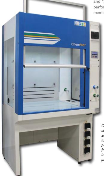
Customized option for handling strong acids at high temperatures are available: from ceramic work surface to internal coating with ceramic panels in monolite IPERGRES; from polypropylene work surface to internal coating with polypropylene panels.
